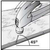
The last rows will not allow the use of the stapler. Manual nailing has to be done on the tongue. Pre drill pilot holes at 45° and drive finishing nail.
