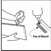
Apply a continuous line of bead of adhesive to the upper part of the grooves' inside edge. Immediately wipe off any excessive adhesive with damp cloth.
