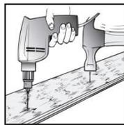
Install the first row of starter board along the chalk line/straight edge. Secure into position with groove-side facing the wall. Drill pilot holes on the board's face near the chalk line and fasten with finish nail.
