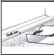
Spread recommended adhesive using notched trowel, from the chalk line/straight edge to approximately the width of two boards.
