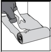
Underlayment may be used for sound insulation and/or for smoothing out slight irregularities of the sub-floor. Do not overlap the underlayment.
