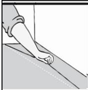
Snap a chalk line from these measured points, parallel to the starter wall and perpendicular to the adjacent wall. While most walls are not square, trim the boards to fit along the adjacent wall.
