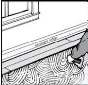
Lay the first row of starter boards along the chalk line/straight edge. Starting from the left corner, secure the boards into position with tongue-side facing the wall.
