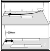
On starting the next row, always make sure to stagger the end joints by at least 12 in (30 cm). Try to use cut piece from previous row to start new row.
