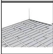
After every 3 rows of boards are laid down, stick strips of masking tape e.g. 3M 2090 Blue Mask™ to hold the boards together to prevent minor shifting or gapping.
