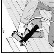
Make sure the starter row is straight and secure before continuing to staple the remaining rows.
