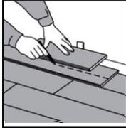
To lay the last row, place a full length floor board directly on top of the last installed row. Measure and cut the correct width by putting a full width scrap board with spacers inserted against the wall.
