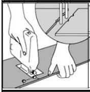
On encountering pipes, ensure the position and diameter of the pipe; drill hole(s) with diameter  $\frac{3}{8}$  in (10 mm) larger. Cut off as shown in the figure and lay the board in place. Apply adhesive to the loose piece and fit it in place.
