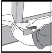
Lay a loose board upside down as a proper height guide against the door jamb. Cut the bottom of the frame off, leaving the required expansion gap allowance.
