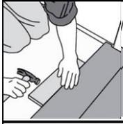
All joints shall have a tight fit. Use tapping block and hammer to tap any gapped joints as necessary. Never hit the floor board directly with hammer.
