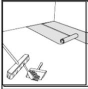
After cleaning the sub floor, roll over the vapor barrier sheet with a minimum 8 in (20 cm) overlap. Unroll the sheet along the longest wall.
