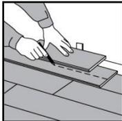
On the far wall, place a full length floor board directly on top of the last installed row. Measure and cut the correct width by putting a full width scrap board.
