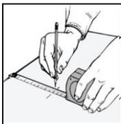
At each end of the starter wall, measure out the width of two boards plus the tongue and expansion gap allowance.
