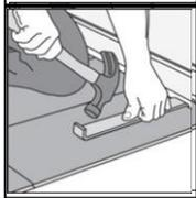
Use pull bar and hammer to tap gapped joints at adjoining wall and door jamb.
